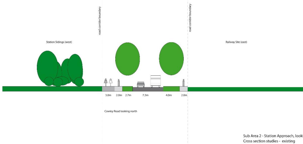
Below: Existing street section
